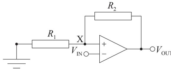
The supply voltages to the operational amplifier are +15 V and -15 V. The resistors have the values  $R_1 = 47 \text{ k}\Omega$  and  $R_2 = 420 \text{ k}\Omega$ .
