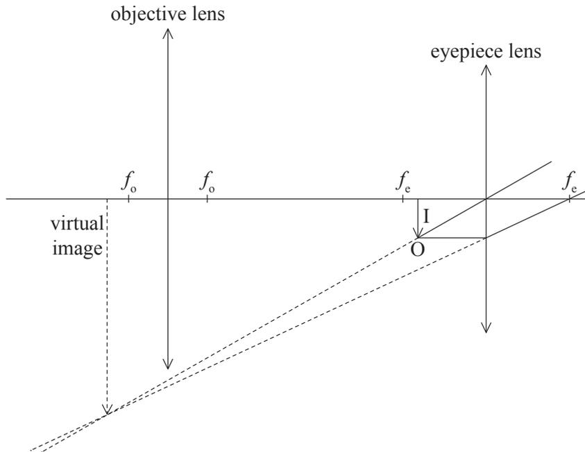
at least two rays from O correctly refracted at eyepiece;
