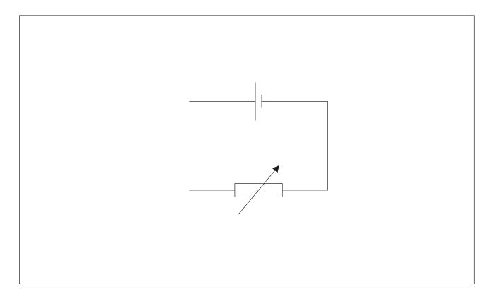
The variable resistor is set to  $1.5\,\Omega$ . When the cell converts  $7.2\,\text{mJ}$  of energy,  $5.8\,\text{mC}$  of charge moves completely around the circuit. The potential difference across the variable resistor is  $0.55\,\text{V}$ .
