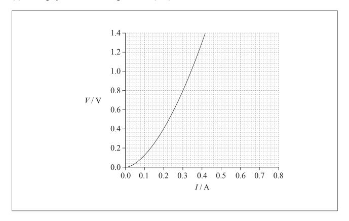
The variable resistor in the circuit in (c) is replaced by this non-ohmic conductor.
