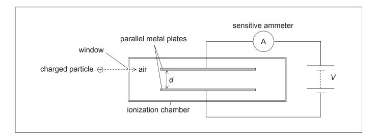
The charged particles enter the chamber through a thin window. They then ionize the air between the parallel metal plates. A high potential difference across the plates creates an electric field that causes the ions to move towards the plates. Charge now flows around the circuit and a current is detected by the sensitive ammeter.
