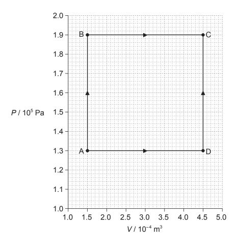
The temperature of the gas at point A is 85 °C. The gas can change its state to that of point C either along route ABC or route ADC.
