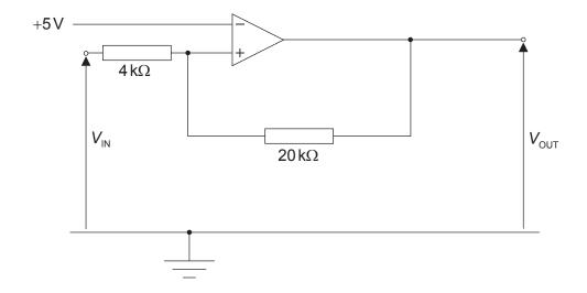
The output of the Schmitt trigger is positive saturation (+15 V) or negative saturation (-15 V). Calculate the input value that will cause the output to switch from -15 V to +15 V.
