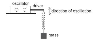
The mass is performing very lightly damped harmonic oscillations. The frequency of the driver is **higher** than the natural frequency of the system. At one instant the driver is moving downwards.
