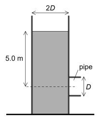
When the pipe is opened, water exits the pipe with speed u and the surface of the water in the tube moves downwards with speed v.
