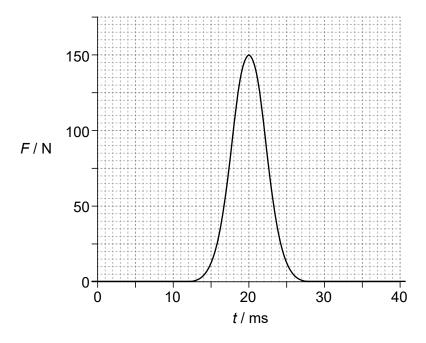
The tennis ball was stationary at the instant when it was hit. The mass of the tennis ball is  $5.8\times10^{-2}$  kg. The area under the curve is  $0.84\,N\,s$ .
