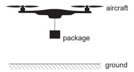
The air is propelled vertically downwards with speed v. The aircraft hovers motionless above the ground. A package is suspended from the aircraft on a string. The mass of the aircraft is 0.95 kg and the combined mass of the package and string is 0.45 kg. The mass of air pushed downwards by the blades in one second is 1.7 kg.
