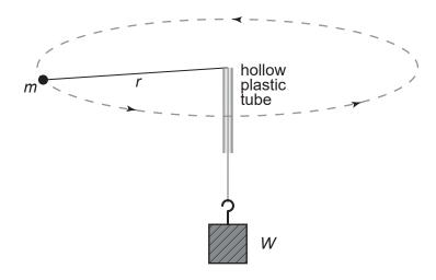
The student collects the measurements of T five times, for weight W. The weight is then doubled (2W) and the data collection repeated. Then it is repeated with 3W and 4W. The results are expected to support the relationship
