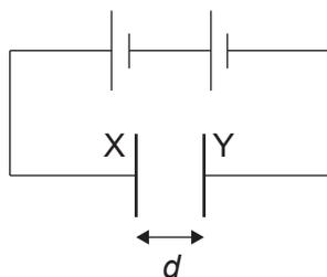
The capacitor has a capacitance  $C$  and a charge  $Q$ . The plates X and Y of the capacitor are a distance  $d$  apart. Edge effects are negligible.
