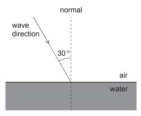
(ii) The speed of sound in air is  $340 \,\mathrm{m\,s^{-1}}$  and in water it is  $1500 \,\mathrm{m\,s^{-1}}$ .
