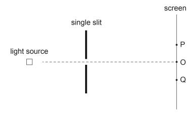
O is the point on the screen directly opposite the slit. P and Q are the first minima on either side of the central fringe of the diffraction pattern.
