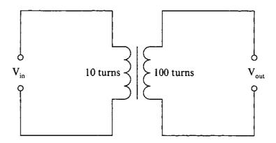
If a 20 V battery is connected to the input terminals then at steady state the voltage output would be
