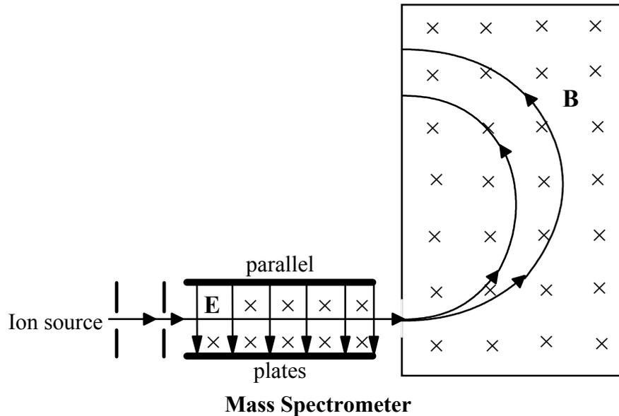
Magnetic deflecting force is the same (same charge and velocity in magnetic field). But mass is greater so acceleration is less, hence more massive ion is not deflected as much, implies larger radius.
