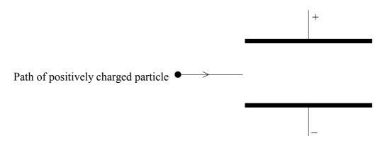
A positively charged particle passes into the region between the plates. Initially, the particle is travelling parallel to the plates.
