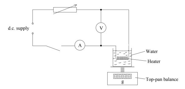
The current was switched on and maintained constant using the variable resistor. The readings of the voltmeter and the ammeter were noted. When the water was boiling steadily, the reading of the top-pan balance was taken and, simultaneously, a stopwatch was started. The reading of the top-pan balance was taken again after 200 seconds and then after a further 200 seconds.
