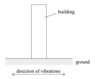
The base of the building vibrates horizontally due to the earthquake.
