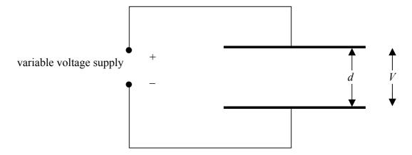
The charge Q on one of the plates is measured for different values of the potential difference V applied between the plates. The values obtained are shown in the table below. Uncertainties in the data are not included.
