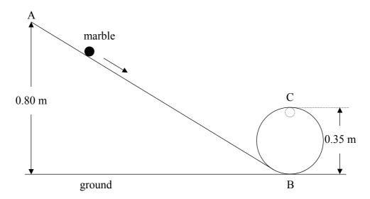
The mass of the marble is 0.050 kg. Friction forces and any gain in kinetic energy due to the rotating of the marble can be ignored. The acceleration due to gravity,  $g = 10 \,\mathrm{m\,s^{-2}}$ .
