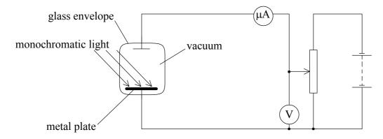
Monochromatic light is incident on the metal plate. The potentiometer is adjusted to give the minimum voltage at which there is zero reading on the microammeter.
