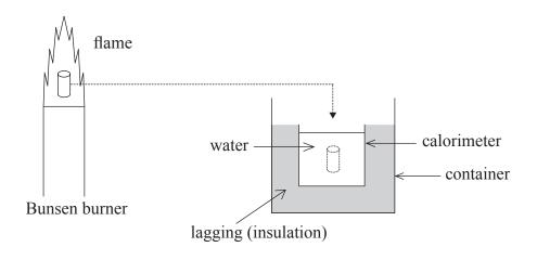
The water into which the metal has been placed is stirred until it reaches a steady temperature.
