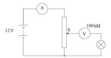
The battery has e.m.f. 12V and negligible internal resistance. The ammeter has negligible resistance and the resistance of the voltmeter is  $100\,\mathrm{k}\Omega$ .
