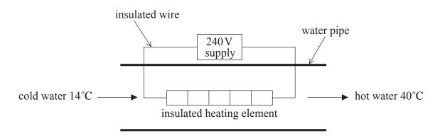
Cold water enters the shower unit and flows over an insulated heating element. The heating element is rated at  $7.2\,\mathrm{kW}$ ,  $240\,\mathrm{V}$ . The water enters at a temperature of  $14\,^\circ\mathrm{C}$  and leaves at a temperature of  $40\,^\circ\mathrm{C}$ . The specific heat capacity of water is  $4.2\times10^3\,\mathrm{J\,kg^{-1}\,K^{-1}}$ .
