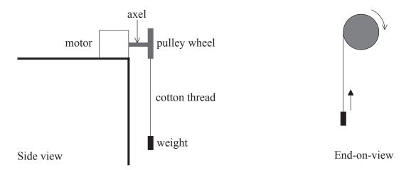
The time taken for the motor to raise the weight through a certain height is measured. It is assumed that the weight accelerates uniformly whilst being raised. The weight of the cotton thread is negligible.
