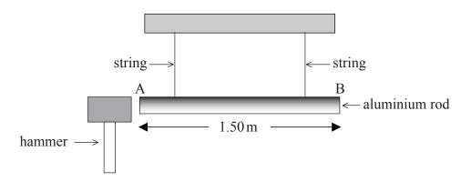
End A of the rod is hit gently with a hammer. As a result, a wave pulse travels down the rod and is reflected from end B. The hammer remains in contact with the rod until the pulse reflected from end B reaches A. This pulse causes the hammer to rebound from the end of the rod.
