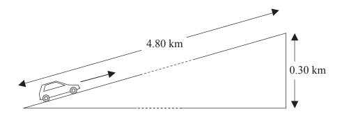
The car moves up the incline at a steady speed of  $16\,\mathrm{m\,s^{-1}}$ . During the climb, the average resistive force acting on the car is  $5.0\times10^2\,\mathrm{N}$ . The total weight of the car and the driver is  $1.2\times10^4\,\mathrm{N}$ .
