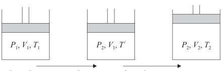
heated at constant volume to pressure  $P_2$  and temperature T' heated at constant pressure to volume  $V_2$  and temperature  $T_2$
