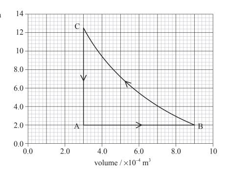
The temperature of the gas at A, the starting point of the cycle, is 17°C.
