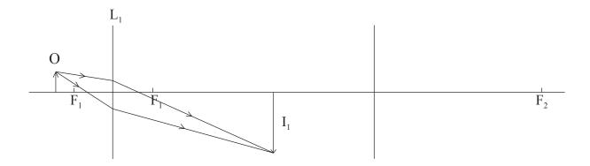
The diagram also shows two rays from the object O to the position of the image  $I_1$  produced in the lens  $L_1$ .
