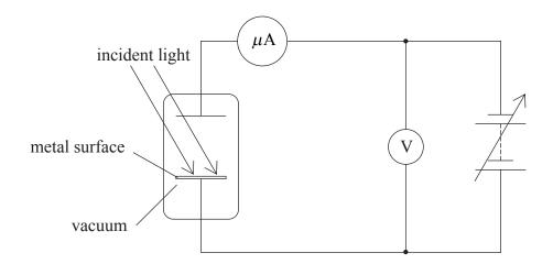
The minimum potential  $V_{\rm S}$  (the stopping potential) necessary to give zero reading on the microammeter is measured for different values of the wavelength  $\lambda$  of the light incident on the metal surface.
