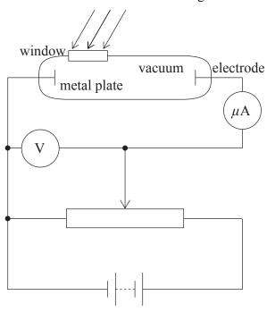
The potential difference V applied between the metal plate and electrode may be varied in magnitude and in direction. This is repeated for different values of intensity for the same frequency of light.
