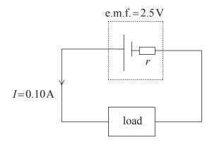
The power dissipated in the load is 0.23 W.
