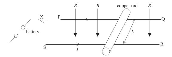
The length of the copper rod between the rails is L. The mass of the copper rod is M. Friction between the copper rod and the rails is negligible.
