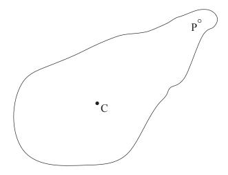
The centre of gravity of the sheet is at point C.
