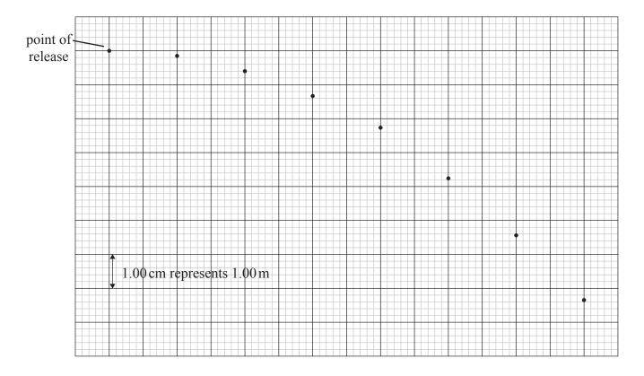
The first photograph is taken at time t=0. Each 1.00 cm on the grid represents a distance of 1.00 m in both the horizontal and the vertical directions.
