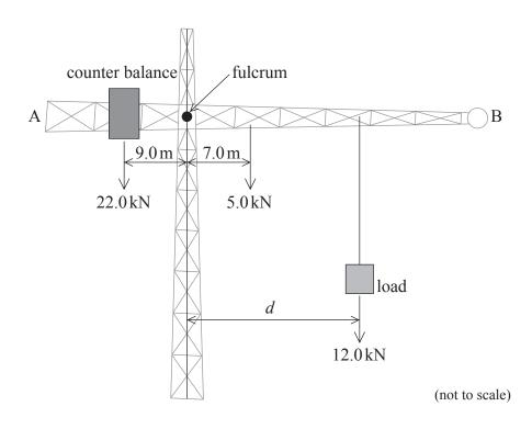
The jib (horizontal section AB) of the crane has a weight of 5.0 kN and its centre of gravity is 7.0 m from the fulcrum. The weight of the counterbalance is 22.0 kN and it acts 9.0 m from the fulcrum. The counterbalance keeps the load and the weight of the jib of the crane in equilibrium.
