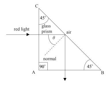
The light undergoes total internal reflection at face BC.
