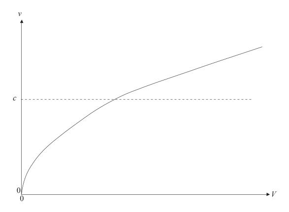
On the graph, draw a line to show the variation with accelerating potential difference V of the speed v of a proton according to relativistic mechanics.
