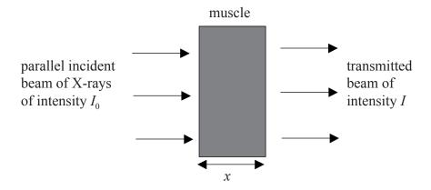
The graph below shows the variation with the thickness x of the muscle of the transmitted intensity I. The units of intensity are arbitrary.
