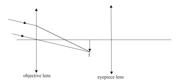
The objective lens has a focal length  $f_{\rm o}$  and the eyepiece lens has a focal length  $f_{\rm e}$ . The objective lens forms an image of a distant object at I. The final image is formed at infinity.
