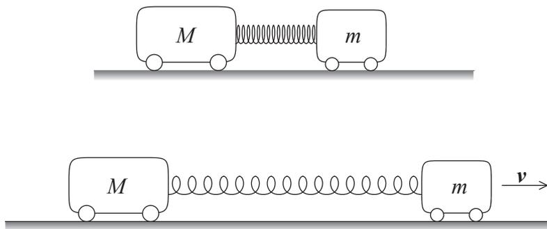
After the carts are released, the cart of mass  $m$  moves with velocity  $v$ . The change in the momentum of mass  $M$  is
