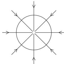
21. In the diagram, a long current-carrying wire is normal to the plane of the paper. The current in the wire  $\otimes$  is directed into the plane of the paper.
