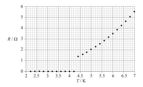
The hypothesis is that resistance is proportional to absolute temperature for temperatures greater than 4.5 K.
