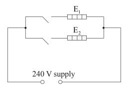
Element  $E_1$  is made from wire that has a cross-sectional area of  $6.8\times10^{-8}\,\text{m}^2$ . The resistivity of the wire at the operating temperature of the element is  $1.1\times10^{-6}\,\Omega\,\text{m}$ .
