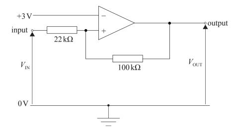
The output of this Schmitt trigger is positive saturation (+13 V) or negative saturation (-13 V).
