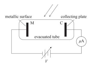
(a) When red light is incident on the metallic surface M the microammeter registers a current. Explain how a current is established in this circuit even though nothing joins M to C inside the tube.
