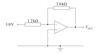
Calculate the output voltage  $\,V_{\mathrm{OUT}}.$
