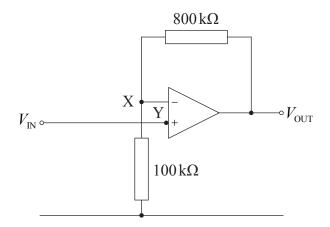
(a) The values of the resistors in the circuit are  $800\,\mathrm{k}\Omega$  and  $100\,\mathrm{k}\Omega$  as shown in the diagram. Calculate the gain of the amplifier.
