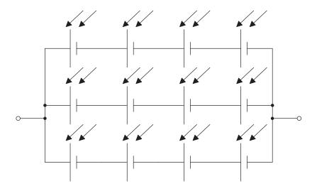
Each cell in the module has an emf of  $0.75\,\mathrm{V}$  and an internal resistance of  $1.8\,\Omega$ .
