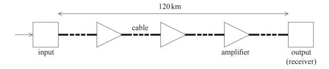
The power of the input signal is 240 mW. The output signal power must not fall below 12 mW.
