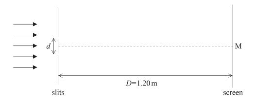
The distance D between the slits and the screen is 1.20 m. The slit separation d is 0.150 mm.
