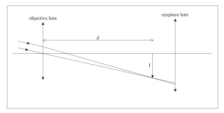
The image I of a star is formed by the objective lens at a distance d from the objective lens. The final image of the star is formed at infinity.
