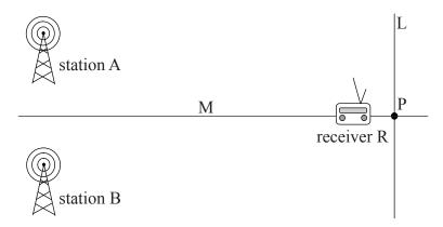
Discuss the variation of the intensity of the radio signal with position as the receiver is moved along line M.
