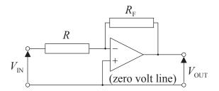
The op-amp operates with a power supply of  $\pm 6.0 \,\mathrm{V}$ . The resistance of  $R_{\mathrm{F}}$  is  $75 \,\mathrm{k}\Omega$  and the resistance of R is  $15 \,\mathrm{k}\Omega$ .
