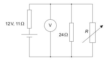
Power supplies deliver maximum power to an external circuit when the resistance of the external circuit equals the internal resistance of the power supply.
