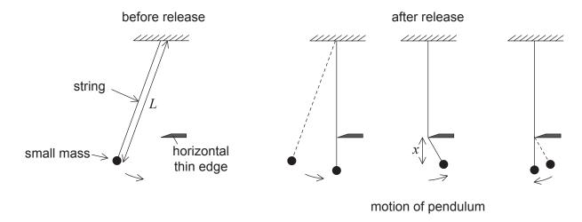
The length L of the string is kept constant during the experiment. The vertical position of the horizontal thin edge is varied to change x.
