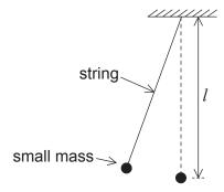
The time *T* taken for the mass to swing through one cycle is given by
