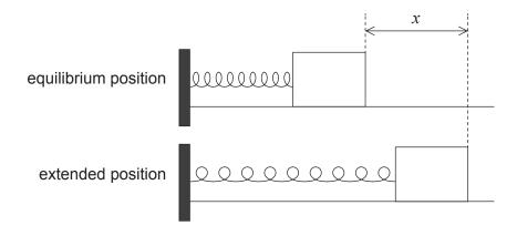
The tension F in the spring is given by F = kx where x is the extension of the spring and k is a constant.
