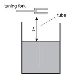
A tuning fork is sounded above the tube. For particular values of L, a standing wave is established in the tube.
