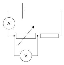
What changes occur in the ammeter reading and in the voltmeter reading when the resistance of the variable resistor is increased?
