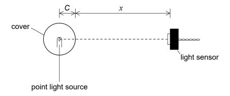
The light source emits radiation with a constant power P and all of this radiation is transmitted through the cover. The relationship between I and x is given by
