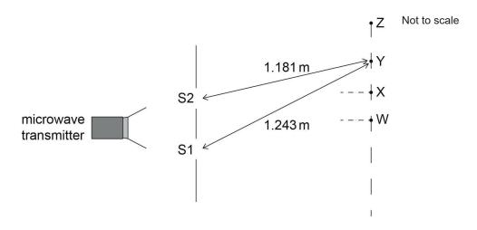
When a microwave receiver is initially placed at W which is equidistant from the slits, a maximum in intensity is observed. The receiver is then moved towards Z along a line parallel to the slits. Intensity maxima are observed at X and Y with one minimum between them. W, X and Y are consecutive maxima.
