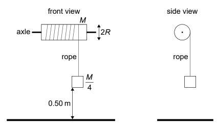
The system is initially at rest and the block is released. The moment of inertia of the cylinder about the axle is  $\frac{1}{2}MR^2$ .
