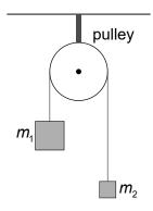
The student calculates the acceleration a of the blocks by measuring the time taken by the heavier mass to fall through a given distance. Their theory predicts that  $a = g \frac{m_1 - m_2}{m_1 + m_2}$  and this can be re-arranged to give  $g = a \frac{m_1 + m_2}{m_1 - m_2}$ .
