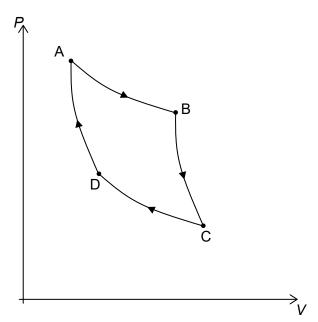
The highest temperature in the cycle is 620 K and the lowest is 340 K.
