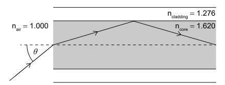
(i) Calculate the critical angle at the core–cladding boundary.
