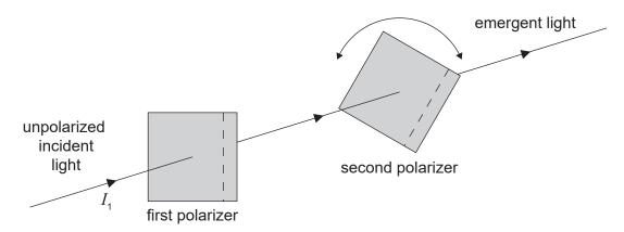
The second polarizer can be rotated to vary the intensity of the emergent light. What is the maximum value of the intensity emerging from the second polarizer?
