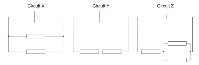
What is the order of increasing power dissipated in each circuit?
