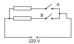
The circuit transfers 1.6 kW when switch A only is closed. The external voltage is 220 V.
