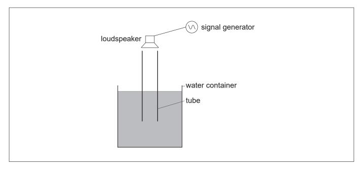
(iii) Between the first and second positions of maximum loudness, the tube is raised through 0.37 m. The speed of sound in the air in the tube is 320 m s<sup>-1</sup>. Determine the frequency of the sound emitted by the loudspeaker.
