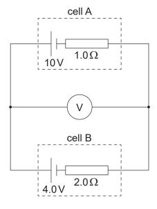
Cell A has an emf of 10 V and an internal resistance of 1.0  $\Omega$ . Cell B has an emf of 4.0 V and an internal resistance of 2.0  $\Omega$ .
