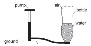
The air-water mixture is called the propellant.
