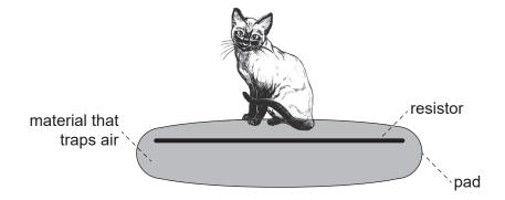
Explain, with reference to thermal energy transfer, why the pad is designed in this way. [3]
