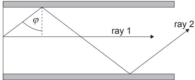
The length of the optical fibre is 1 km. Show that the time delay between the arrival of the two rays at the end of the optical fibre is about 37 ns.
