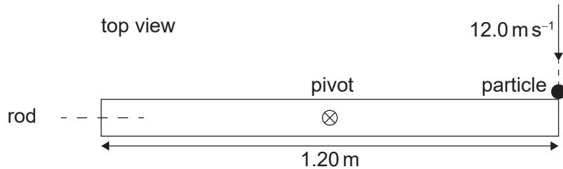
A particle of mass 0.200 kg moving with speed  $12.0 \text{ m s}^{-1}$  collides with and sticks to one end of the rod.
