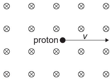
In the reference frame in which the magnetic field is at rest, the proton experiences an initial magnetic force  $evB$  upwards.
