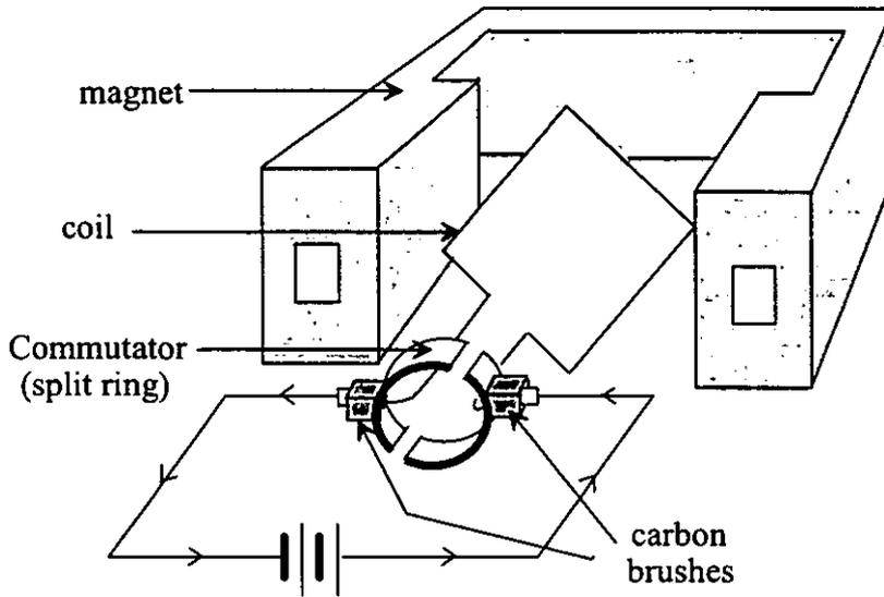
(a) With a battery connected as shown, the motor coil is observed to rotate **clockwise**.
