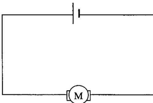
A 6.00 kg mass is fastened by a string to the shaft of the motor. The mass is raised slowly at a constant speed to a height of 0.80 m in 24 s. During this time, the readings of the voltmeter and ammeter are 6.0 V and 0.50 A respectively.
