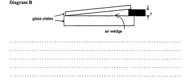
(b) This arrangement can be used to measure small distances, much less than the thickness of a sheet of paper. A sample whose thickness, t, is to be measured is shown in the figures above. Explain how t can be determined.
